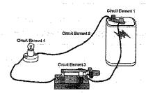
Electricity flows through the closed circuit. When the circuit is closed, the light bulb will light up.
